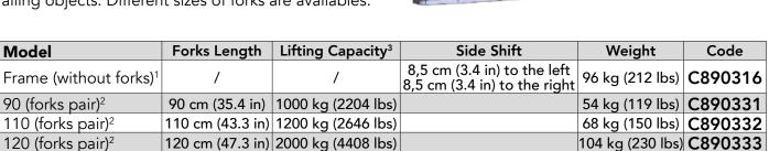
(¹) C890331 or C890332 or C890333 required - (²) C890316 required - (³) verify the lifting capacity of the machine
