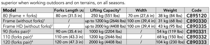
(1) C890331 or C890332 required - (2) C890331 or C890332 or C890333 required - (3) C890330 or C890335 required - (4) C890335 required - (5) verify the lifting capacity of the machine
